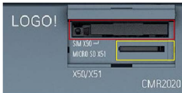
Figure 4-3 Slot for the micro SD card (yellow rectangle)
